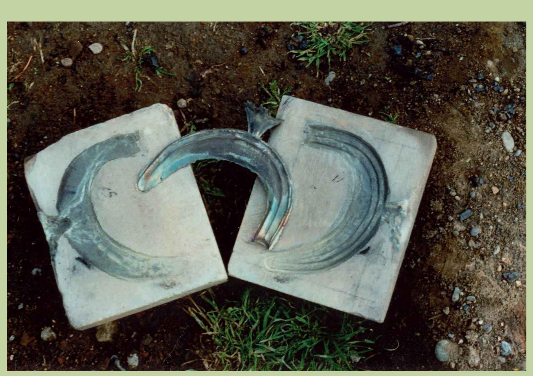
The cast is taken out of the mould and finished.
