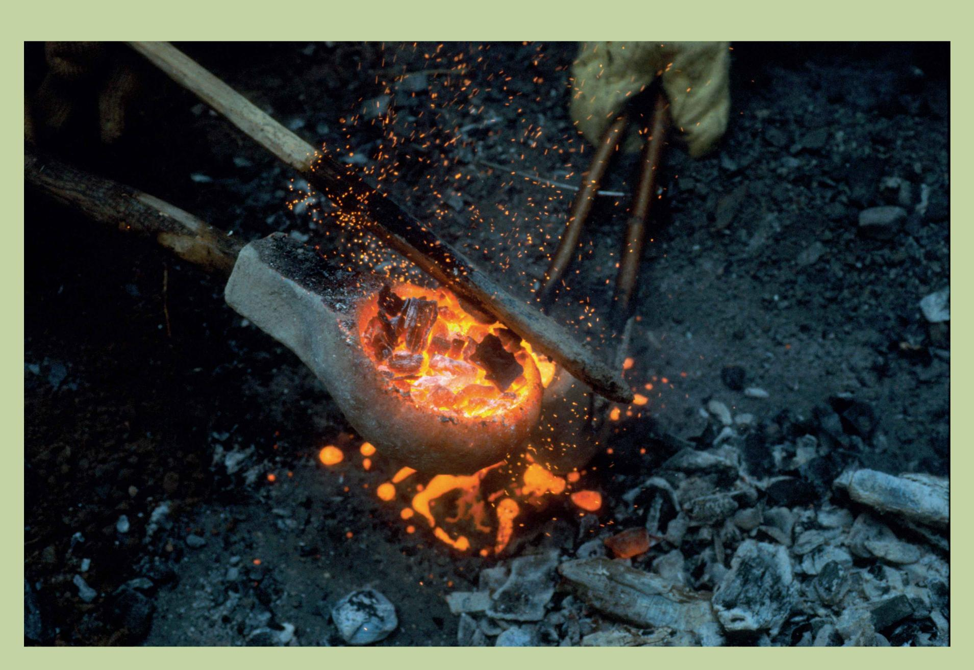
The bronze, which has melted at a temperature of just under 1000°C, is poured into the mould.
